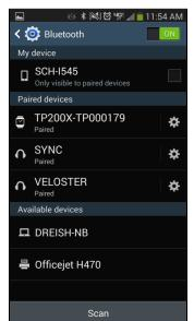
Upon first connection, enter PIN 1234 or 1111 to connect to TruPulse device. Different Android devices behave differently. If prompted to accept a "Passkey" simply click "OK."
